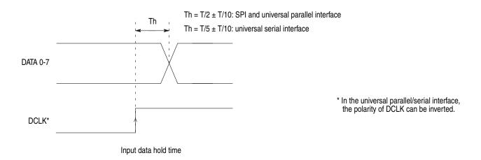
Figure A-1: Timing diagram of the SPI and universal parallel/serial interfaces
