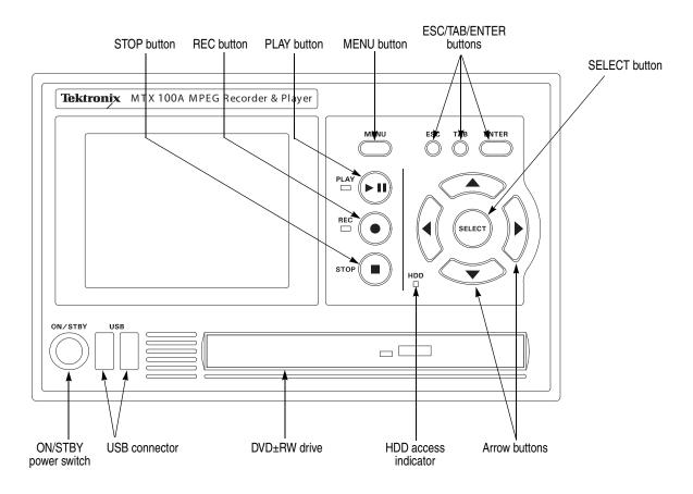
Figure 2-1: MTX100A front panel
