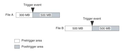
■ If a second trigger event occurs while the posttrigger area is filled with data, the second trigger event is ignored.
