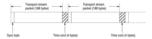
Figure 3-40: Partial transport stream
