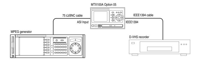
Figure 3-38: Connection example for ASI → EEE1394 conversion
