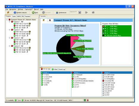
Figure 2-16: Transport stream display from an MPEG test system
