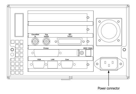
Figure 1-1: Rear-panel power connector
