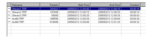
■ If you set a Start Time (for example, 2005/2/10 15:00:00) in the Play Properties dialog box for an individual stream, the start date/time of all subsequent streams are changed. This does not affect the preceding streams.
