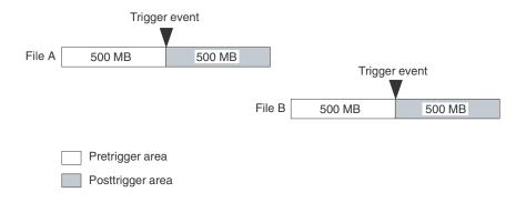
If a trigger event occurs while the pretrigger area is filled with data, the pretrigger area becomes smaller than the specified size. However, the posttrigger area stays the specified size. In this case, File A is smaller than the specified size.
