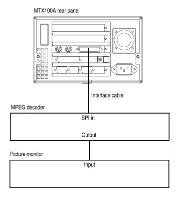
Figure 1-4: Equipment connection for the functional check
