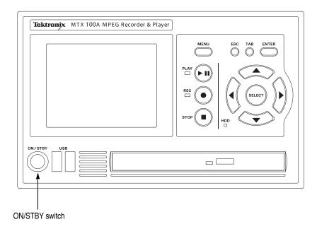
Figure 1-2: Front-panel ON/STBY switch
