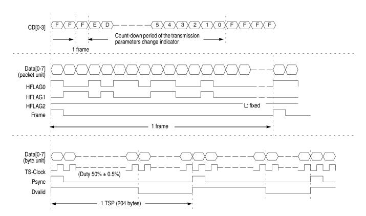
Figure D-1 shows the timing relationship of the signals on the Universal In/Out connector.
