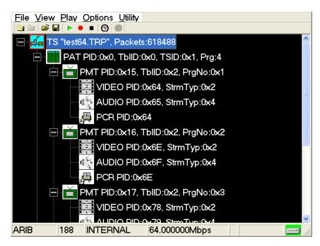
Figure 2-14: Hierarchy view of the transport stream file
