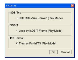
**Data Rate Auto Convert (Play Mode):** Sets whether to set the clock rate automatically when the ISDB-TSB file is loaded. Press the TAB button repeatedly to select this item, and then press the SELECT button to toggle the check box on (checked) or off (not checked). When it is checked, the clock rate is automatically set to (2048/1701) x 27 MHz and the elementary stream rate becomes constant regardless of the Fixed ES Rate setting.
