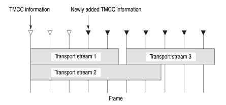
This illustration shows the placement of the new TMCC information and the transport stream 3 when they are multiplexed after the transport stream 1. The new TMCC information is inserted two frames before the location in which the new transport stream is inserted.
