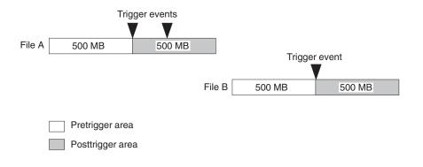
**NOTE.** If the trigger position is set to 0 (%), both files are created whenever a trigger event occurs.
