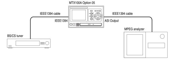
Figure 3-39: Connection example for IEEE1394—ASI conversion
